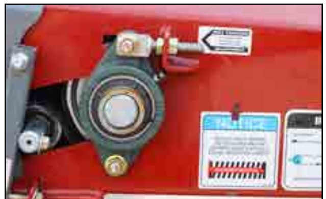
Fig 27 - Conveyor belt adjustment
