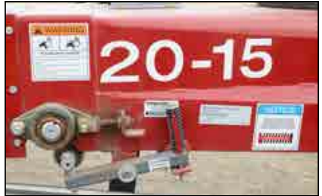
Fig 21 - Swing belt adjustment
