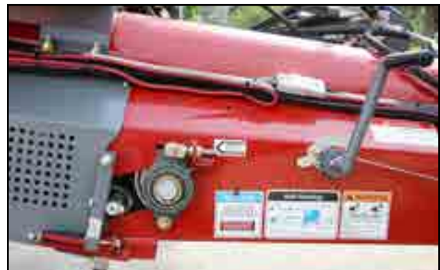
Fig 20 - Drive box belt adjustment
