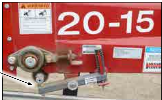
Fig 26 - Swing pinch roller belt adjustment
