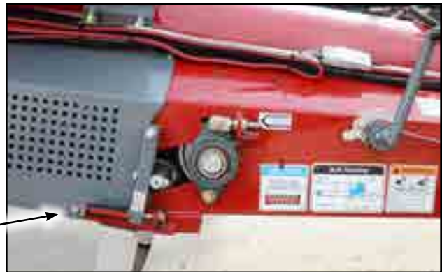
Fig 25 - Main conveyor pinch roller belt adjustment
